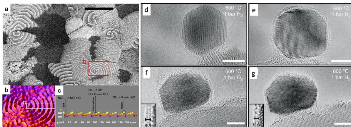
**Figure 1:** (a-c) Contrast variations caused by propagating chemical waves as revealed by in-situ SEM during NO<sub>2</sub> hydrogenation on a polycrystalline Pt foil [1]. Examples of in-situ TEM are shown in panels (d-g): A platinum particle on a titania support in the first exposure to H<sub>2</sub> at 600 °C (d, e) and the subsequent atmosphere change to O<sub>2</sub> at 600 °C (f), and back to H<sub>2</sub> (g). Scale bar: 5nm [2].
