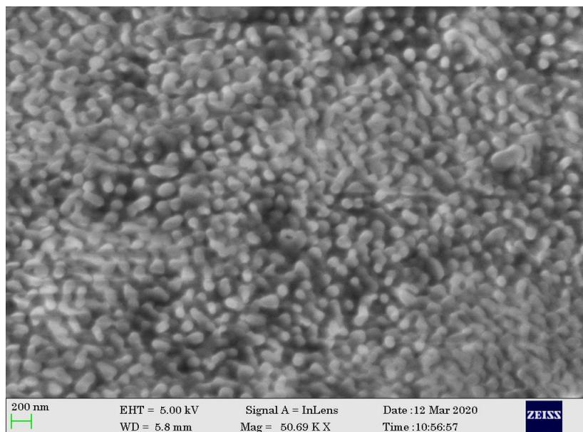
**Figure 1.** Scanning electron micrograph of Ag(0.5 wt%) doped YAG
