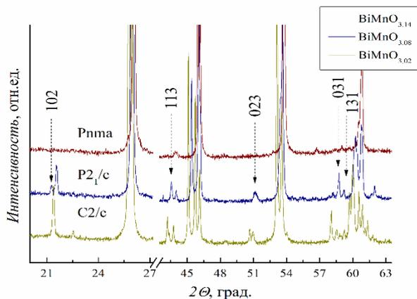
Fig.1. Diffraction patterns of the ceramics  $\text{BiMnO}_{3+d}$  ( $d = 0.02, 0.08, 0.14$ ); reflections characteristic for different structural phases are marked.
