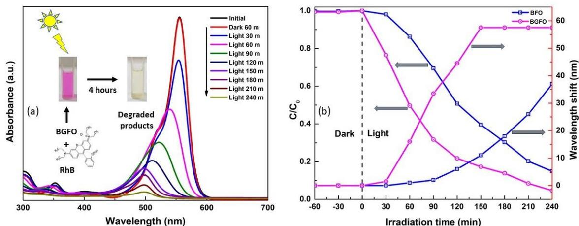
Fig: (a) Spectral changes during the degradation of RhB dye in the presence of BGFO nanoparticles under solar irradiation and (b) A plot of degradation (%) vs irradiation time (min) for BFO and BGFO nanoparticles (black Y axis) and corresponding wavelength shifts in the absorbance band of RhB (red Y axis).
