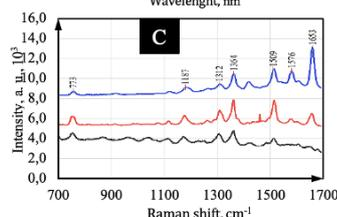
Figure 1 – SEM-image of Ag/Ni/macroPS surface (A), reflectance spectrum (B) and SERS-spectra of Rhodamine 6G  $10^{-6}$  M
