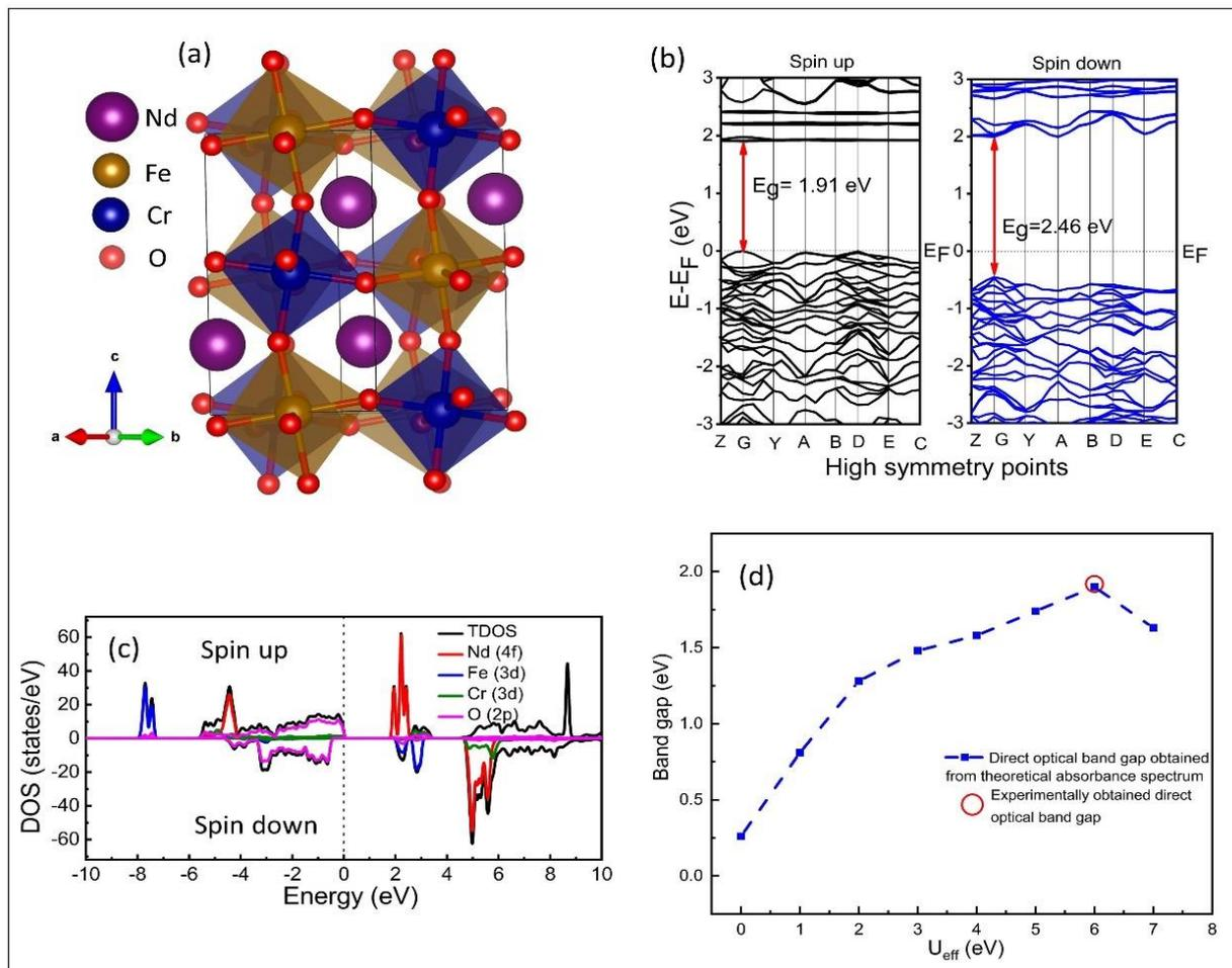
Fig. (a) Schematic representation of the  $\text{Nd}_2\text{FeCrO}_6$  monoclinic unit cell with its (b) band structure and (c) total density of states and partial density of states of Nd-4f, Fe-3d, Cr-3d and O-2p orbitals for  $U_{\text{eff}} = 6$  eV. (d) Variation in theoretically calculated direct optical band gap as a function of  $U_{\text{eff}}$ . The red circle in fig (d) represents the experimentally obtained optical band gap value.
