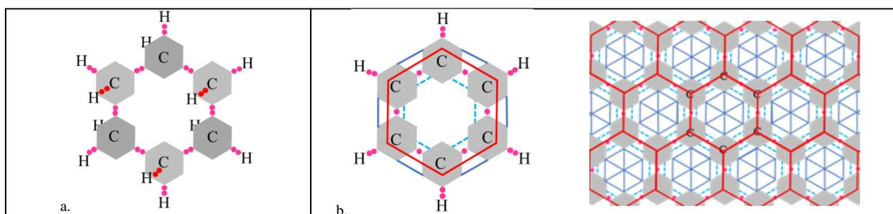
**Fig. 1.** Colors indicate binding plans and single line indicates an electron of the  $\pi$  bond equally shared between two atoms. a) Cyclohexane: bond length C - C  $\approx (\sqrt{3}l) / 2 \approx 153.20$  pm, bond angles  $\approx 109.5^\circ$ . b) Benzene and graphene: bond angles  $\approx 120^\circ$ , bond length  $\approx (\sqrt{2}l) / (\sqrt{3}) \approx 141.98$  pm but the C-C bond in benzene is stretched only in two directions which reduces its calculated value.
