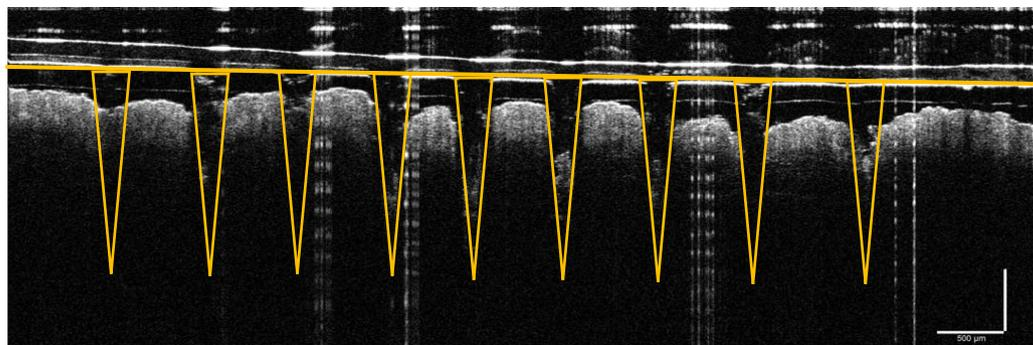
**Figure 3 - B-Scan OCT image of microneedle array in skin - microneedle shape highlighted by yellow**
