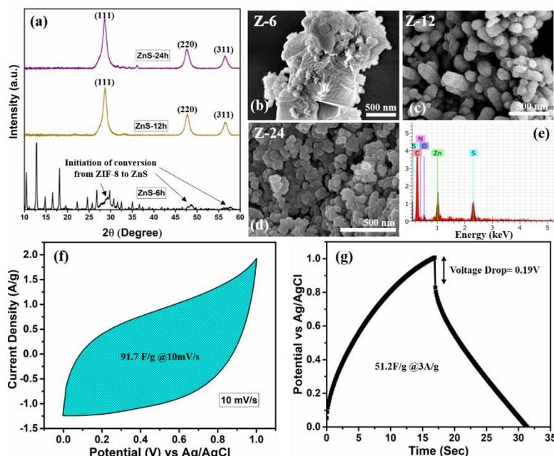
**Figure 1** (a) XRD, FESEM of (b) Z-6, (c) Z-12, (c) Z-24, (d) EDS of Z-24, (f) CV, and (g) GCD of Z-24.
