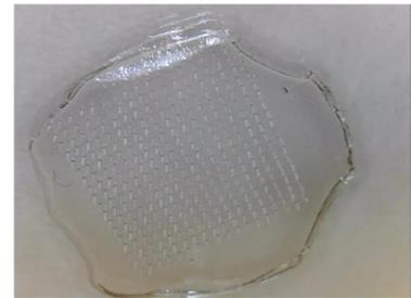
**Figure 2 - Microneedle array structure consisting of 324 needles of height 750  $\mu\text{m}$ , base diameter 200  $\mu\text{m}$ , tip diameter 10  $\mu\text{m}$  and centre-to-centre spacing of 600  $\mu\text{m}$**
