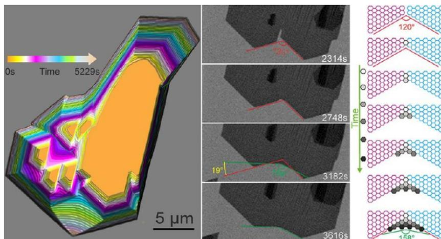
**Figure 1:** Although the scanning electron microscope does not provide in-plane atomic resolution, it is possible to abstract atomistic details about the coalescence behaviour of graphene islands: Analysis of the temporal evolution reveals the underlying processes that lead to the formation of fast growing growth-fronts in seamless coalescence.
