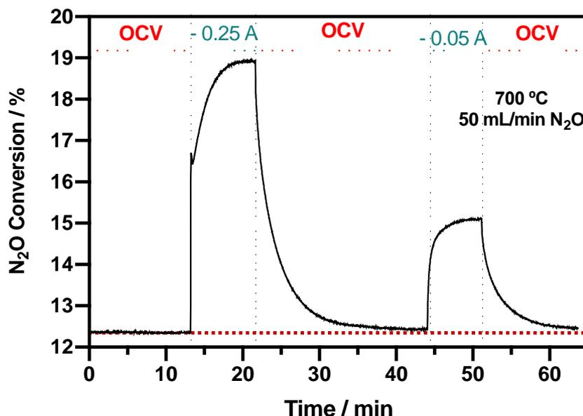
Figure 1 – N<sub>2</sub>O conversion as function of time under polarization (-0.25 and -0.05 A) and OCV conditions.
