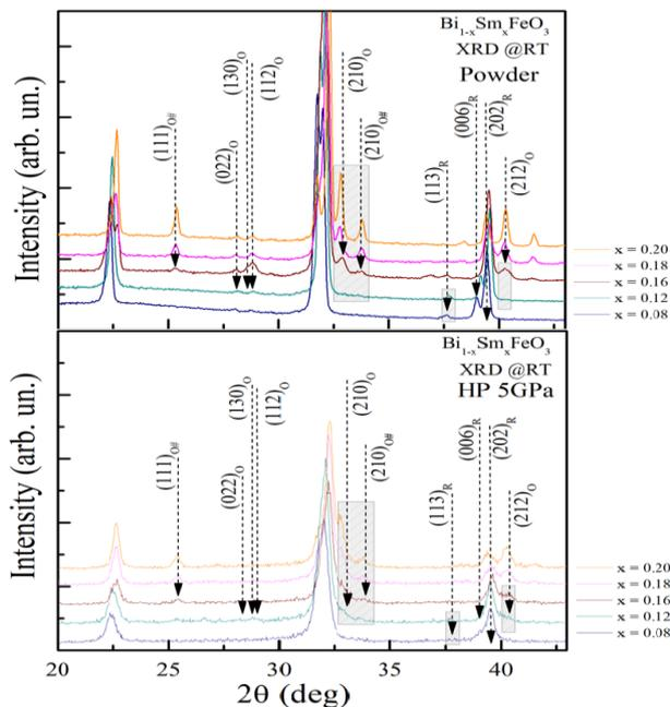
Fig.1. X-ray diffraction patterns of Bi<sub>1-x</sub>Sm<sub>x</sub>FeO<sub>3</sub> (x = 0.08, 0.12, 0.16, 0.18, 0.20) for powders (upper) and tablets obtained after high pressure (5 GPa).
