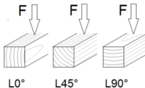
**Figure 1.** The direction of load in relation to annual growth ring orientation [4].
